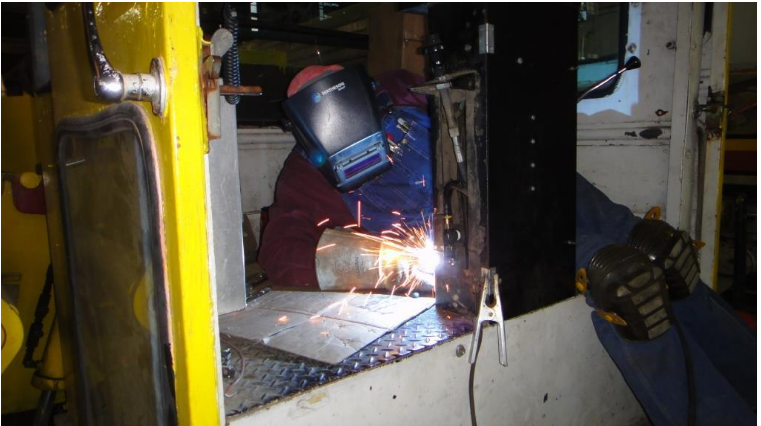
Cliff welds the ballast regulator's console stand back together
